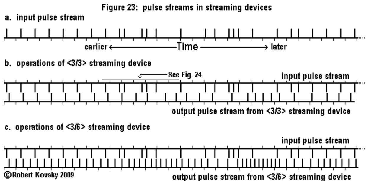
Fig 23.c shows the stream of output pulses of the  $\langle 3/6 \rangle$  streaming device with the same input pulse stream as that shown in previous images. The output pulse stream still correlates to the input pulse stream but with about half the period or about twice the average frequency of pulses.
