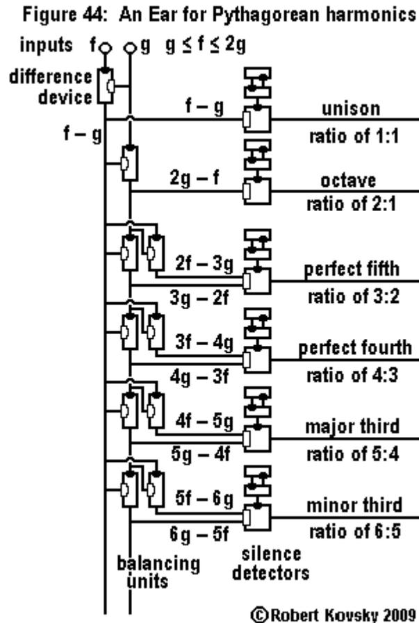
If  $2f-3g \geq 0$ , only the  $f-g$  signal is active in the last three stages of the Ear. The  $f-g$  signal
