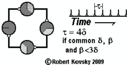
Figure 2 shows four primal timing devices assembled into a “4-cycle.” It is representative of a class of assemblies called n-cycles or, simply, “cycles.” When a 4-cycle is running, each projection carries the signal denoted in the “Time” chart, namely, a sequence of pulses.
