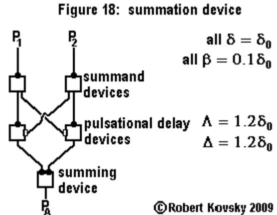
The delays operate so that the frequencies of the pulse streams are, indeed, summed at the summing timing device. If the frequency of  $P_1$  is “20 pulses per second” and the frequency of  $P_2$  is “12 pulses per second,” the frequency of  $P_A$  is “32 pulses per second.”
