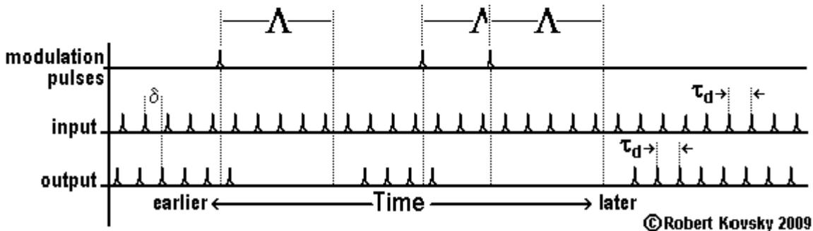
Figure 12.b shows the operations of the “gate normally open” gate timing device. An input pulse leads to a primal, delayed output pulse when “the gate is open” but the output is silent when “the gate is closed.” A modulation pulse closes the gate for a period of  $\Lambda$ , the “modulation period.” The gate is closed as to input pulses arriving after the arrival of the modulation pulse; there is no interruption of a response process initiated prior to the arrival of the modulation pulse.
