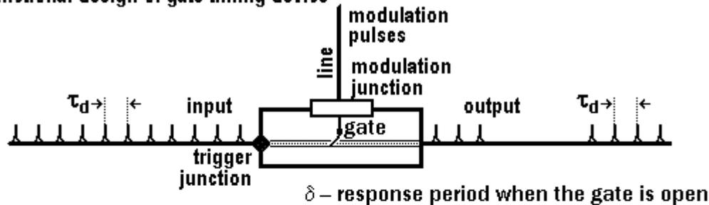
**b. operations where modulation pulse "closes the gate" ("gate normally open")**
