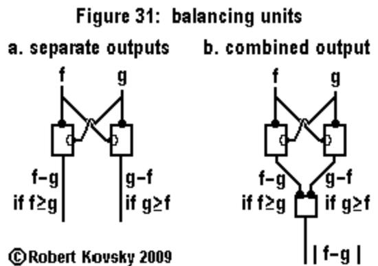
Figure 31.a shows a balancing unit with separate outputs. Suppose that the frequency of pulses through  $f$  is greater than that of those through  $g$  and, therefore, that the  $f-g$  output is active while the  $g-f$  output is silent. Then suppose that the frequency of pulses through  $g$  is gradually increased. When  $f=g$ , both outputs are silent. As  $g$  continues to increase, the  $g-f$  output is
