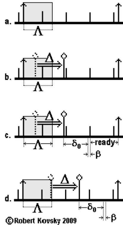
For the activity in Fig. 20.d, the total time before the summing device returns to the ready condition, after having been triggered by the pulses from  $P_1$  and  $P_2$ , is the sum:  $\Lambda + \Delta + \delta_0 + \beta$ . This is shown graphically in Fig. 20.d.
