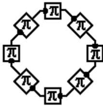
The delay device serves as a memory device. Recall the “cycle” of primal timing devices (Figure 2); the cycle form can be adapted for use of the larger device, as shown in Figure 40. In applications, a cycle of  $n$  delay devices can maintain a “store” of  $n$  pulse bundles, where the pulse bundles might be independent, sequenced or related to one another. The period of activity in the device is  $8\pi$  and continues indefinitely.
