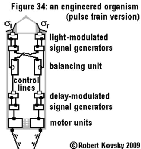
When there is balance, the output of both sides of the balancing unit is a null signal, a condition called “internal silence.” Then, the organism is “heading for the light,” assuming there is a light. If a light is moving from one side to the other, the organism will “follow the light.” The organism acts so that any light becomes “centered” between the sensors. There is a centerpoint of operations around a balanced condition, called “centerpoint balancing.”
