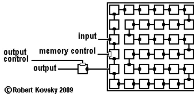
**b. sample pulse bundle for 36 unit delay/memory device**
