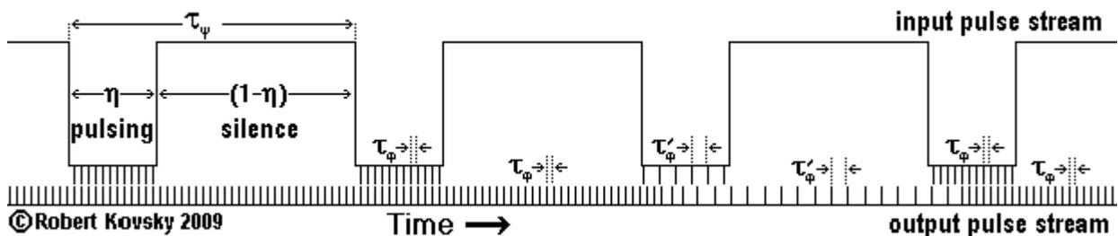
The  $\tau_{MAX}$ -modified streaming device converts input pulse bundles into a continuous output pulse stream made up of segmented output pulse trains with continuous transitions, a highly regular signal. In the modified <3/3> streaming device, each segment in the output pulse stream has a fixed pulse period based on the average occurring in the most recent bundle. Near the beginning of an input pulse bundle, the pulse period of the output stream adjusts to the input pulse periods.
