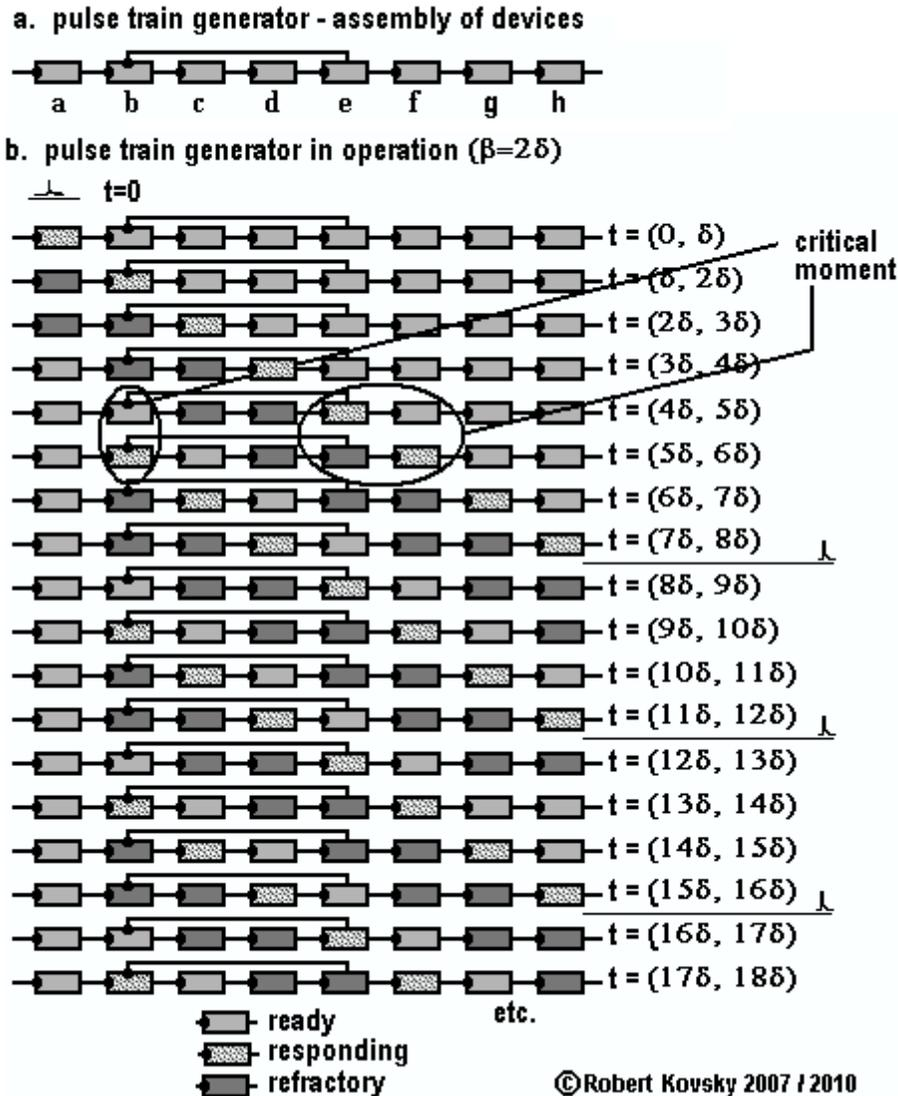
Figure 5.b shows what happens after a single pulse triggers the pulse train generator. For the first several clock ticks, the activity in Figure 5.b is like that shown in Figure 2. The "critical moment" in Figure 4.b occurs at  $t=5\delta$  when timing device e discharges two pulses; one pulse
