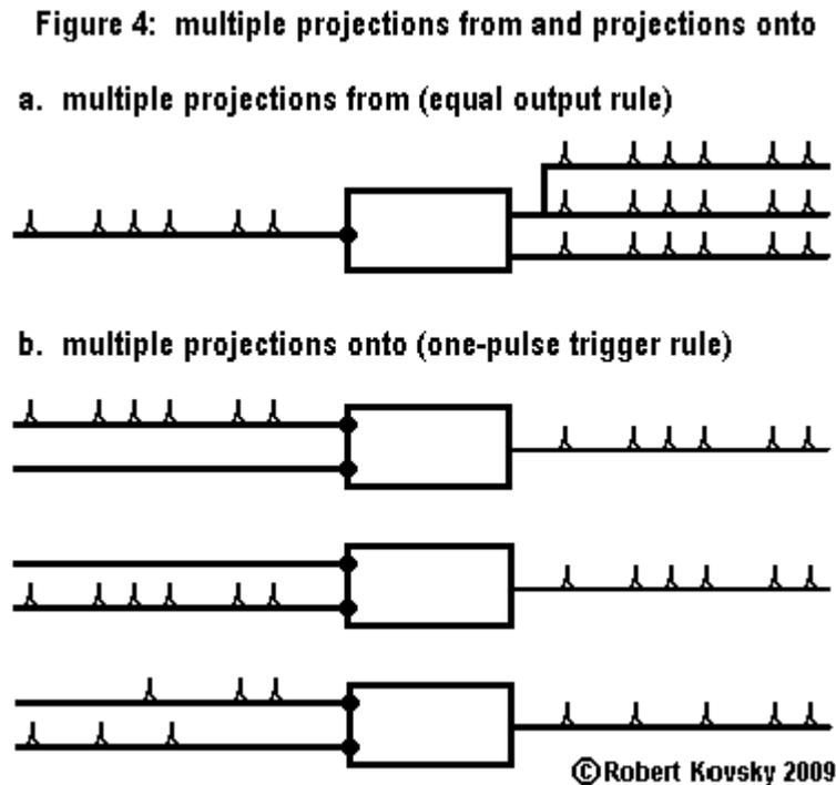
Timing devices with multiple projections onto maintain the operating principle that an input pulse has no effect on device operations unless the device is ready. After the response clock has started and until the timing device returns to a ready condition, the timing device is unresponsive to input pulses arriving through any projection onto.
