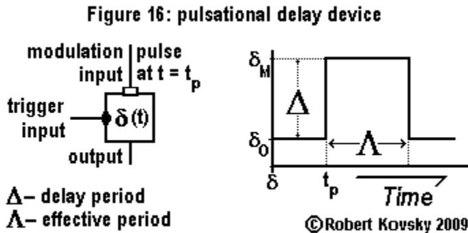
A pulse arriving at the modulation input of the device changes the responding period  $\delta$  for an “effective period” of time,  $\Lambda$ . Normally, the response period is  $\delta_0$  but it is lengthened for the effective period. If a modulation pulse arrives at  $t = t_p$ , and another pulse arrives at the trigger input at any time between  $t_p$  and  $(t_p + \Lambda)$ , the response period will be  $\delta_M = \delta_0 + \Delta$ , adding a “delay period”  $\Delta$ .
