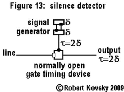
The gate in the silence detector, normally open, stays open so long as “the line is silent,” meaning that there is no signal on the line. While the gate is open, the output is a pulse train produced by the pulse train generator.
