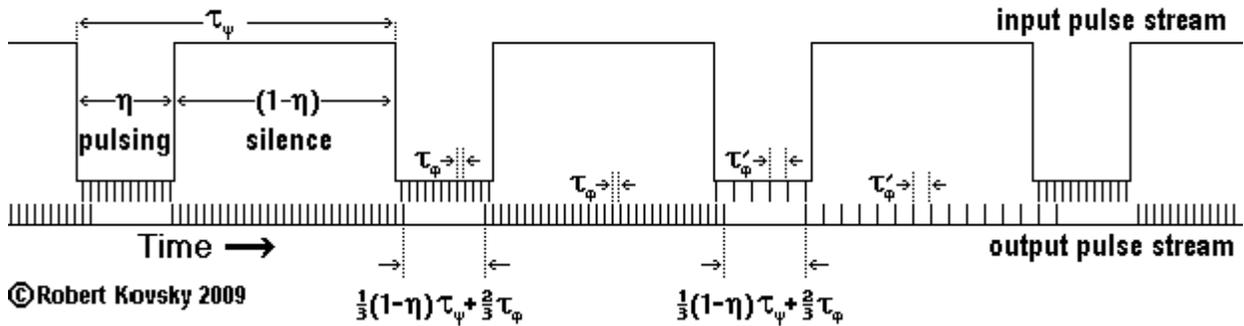
A prominent feature of the output pulse stream in Fig. 25 is the large silent period that occurs during each input bundle. Each large silent period in Fig. 25 is the same size,  $\frac{1}{3}(1-\eta)\tau_\psi + \frac{2}{3}\tau_\phi$ . The large period occurs because the “silent” part of the pulse bundle –  $(1-\eta)\tau_\psi$  – is treated like a period between pulses by the algorithm.
