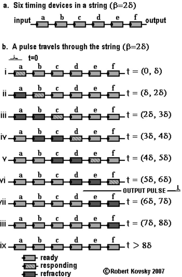
Figure 3.b.ii. shows the conditions between  $\delta$  and  $2\delta$ . As time passes from  $t<2\delta$  to  $t>2\delta$ , timing device b discharges a pulse and changes to the refractory condition. The pulse discharged by timing device b triggers the response process in timing device c and starts its response clock, establishing conditions shown in Figure 3.b.iii. Timing device a remains in the refractory condition until  $t=3\delta$  ( $=\delta+\beta$ ), when it again becomes ready.
