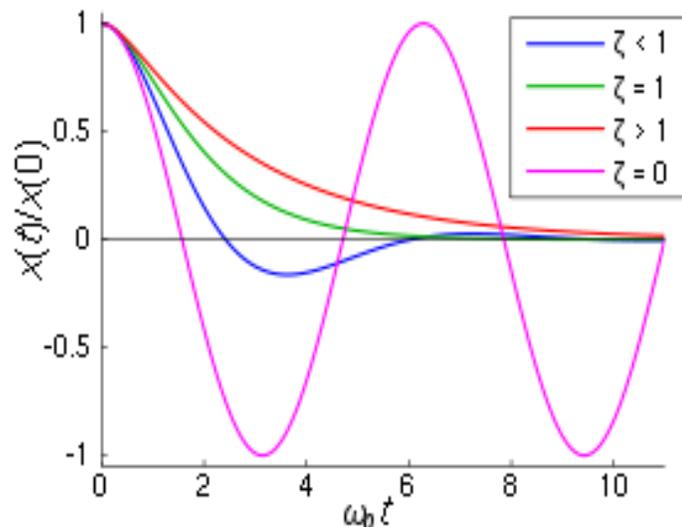
As mentioned in Wikipedia, a mechanical door-closer may have a “damped spring” to return a door to the closed position after being opened. Critical damping provides the fastest closing that avoids having the door bang into the door-frame. Some door-closing devices have an adjustment to make it easier to achieve this standard of performance.
