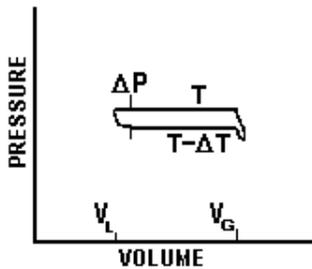
Fig. 45–4. Pressure-volume diagram for a Carnot cycle with a condensable vapor in the cylinder. At the left, the substance is in the liquid state. A quantity of heat  $L$  is added at temperature  $T$  to vaporize the liquid. The vapor expands adiabatically as  $T$  changes to  $T - \Delta T$ .
