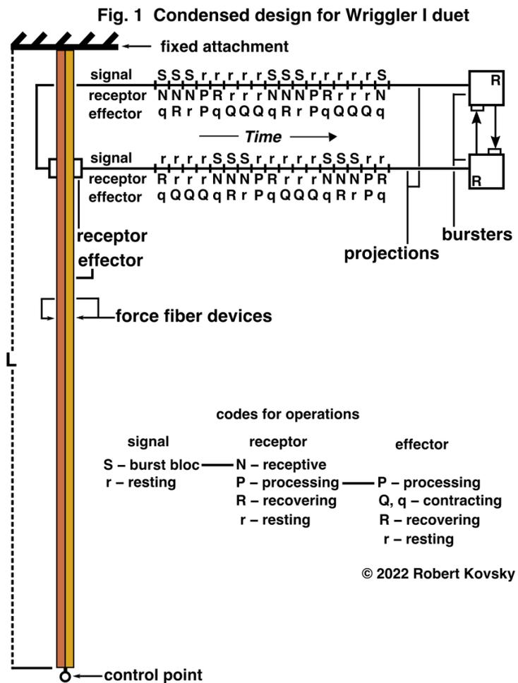
Bursters repeat a signal until it is changed by the researcher. Driven by repeating signals, alternating twitching and ramping forces overlap and combine to produce a steady force, which can be varied. See the wriggler project, Fig. 7, p.20.
