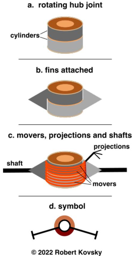
The new version of the spinal hub joint, like the original version, resembles the hub of a bicycle wheel. (Fig. 7.a.) In the new version, two identical cylinders rotate smoothly around a common axis. The central hole is reserved for brachial parts. (See the metamorphosis project at 29 and the wriggler project at 36.)
