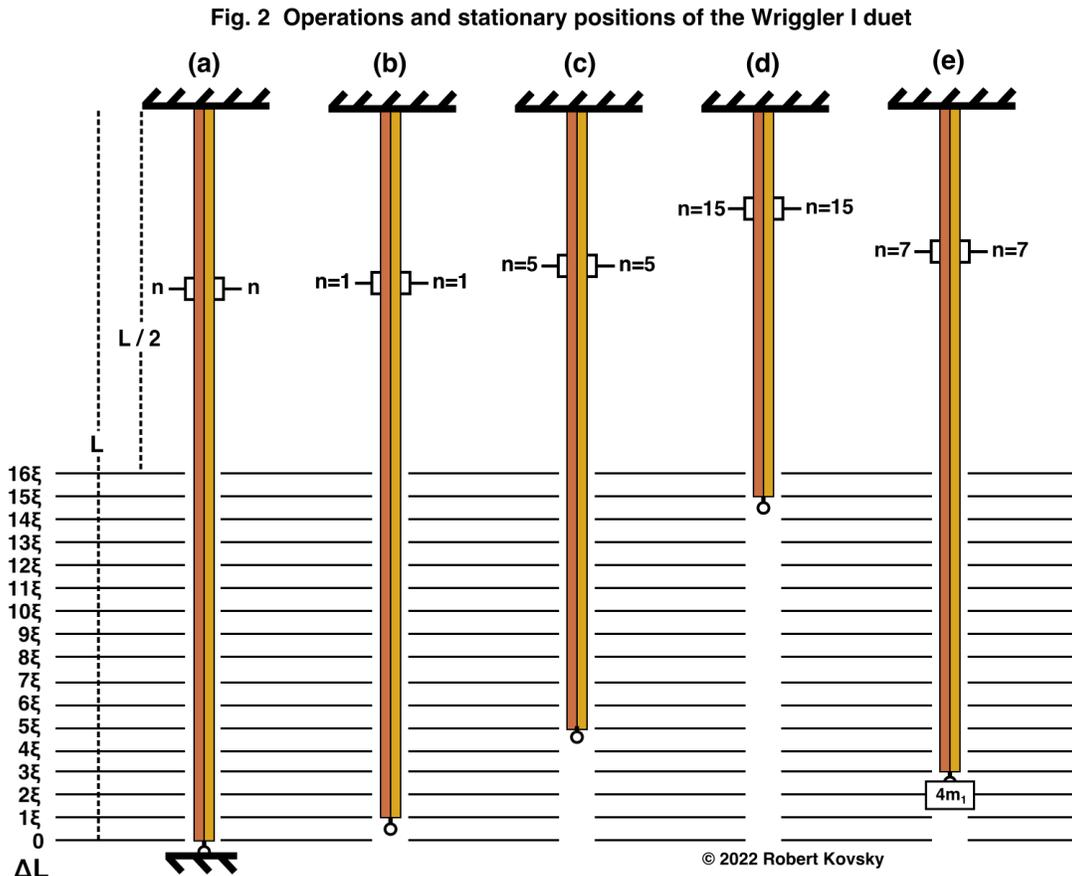
The first force rule is shown in Fig. 2(a). The control point is fixed and the duet is held at full length  $L$ . When steady signals carry bursts with  $n$  pulses, the device produces a steady force of  $F = nF_1$ , where  $F_1$  is the strength of the force produced when  $n = 1$ . There is a variable internal tension but no movement. Force devices with different strengths have parallel repertoires.
