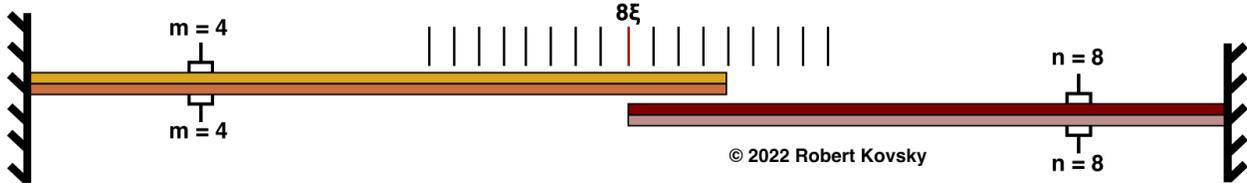
The foregoing constructions are summarized by stating rules for stationary positions of the opposing duet design in terms of drive signals (m,n). Operations require that  $m+n \geq 16$ ; lower drive signals are unworkable. If  $m+n=16$ , no tension is held in the system. Generally, tension  $\tau$  is maintained at  $\tau = \frac{1}{2}(m+n-16) \times F_1$ .
