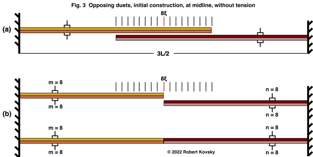
In Fig. 3(b), duets are driven by pulse signals  $(m,n) = (8,8)$ . The length of each duet contracts until the force is 0, occurring when  $\Delta L=8\xi$ . The two loose ends of the duets can be "matched" or juxtaposed; and the surfaces can be attached, glued or otherwise joined sufficiently to withstand operating tensions and impulses. This is the initial stationary position in the repertoire of the opposing duet design.
