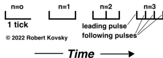
The first pulse in the signal, called the *leading pulse*, starts the device clock but does not modify the strength of the ensuing twitch or pulse burst produced by the receiving device. One to three *following pulses* strengthen the ensuing twitch or burst in equal steps. As shown below in Fig. 13, following pulses are timed so that intervals of time between pulses are identical and the final pulse occurs exactly one tick after the leading pulse.
